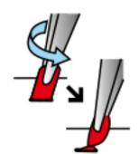
Tab thru hole connection:insert tab thru hole then twist it
